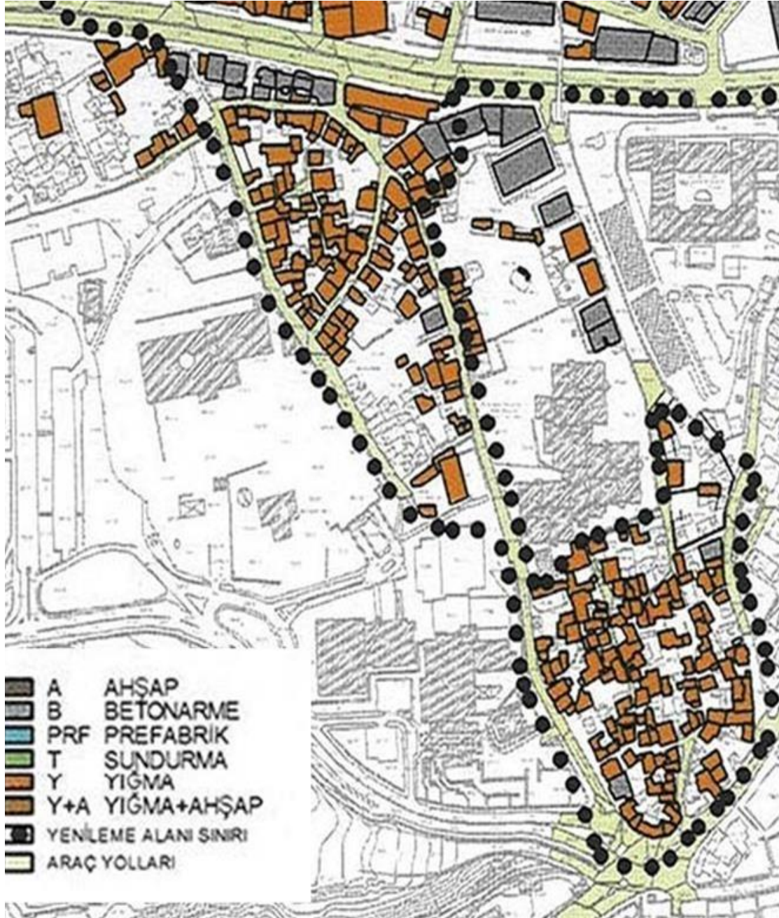
Figure 3.12: Analysis of Structural Systems and Materials of Buildings in the study area before the Rehabilitation Project (Metropolitan Municipality Archives, 2006, access date: 2020)
