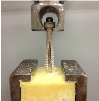
Fig. 2 Photograph of tested sample after static pullout test according to ASTM F543
