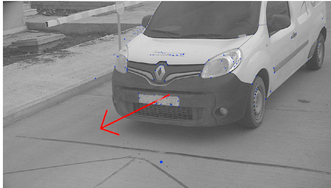
Fig. 4. Resultant motion (red line) and feature locations (blue dots)
