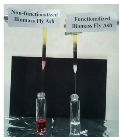
Figure 14. Photograph of columns packed with the A-BFA and BFA-APTES adsorbents. 200 ppm aqueous solution of ARS dye was passed through both the columns. The water coming out of the columns was collected in glass vial for spectrophotometric estimation of the dye content.
