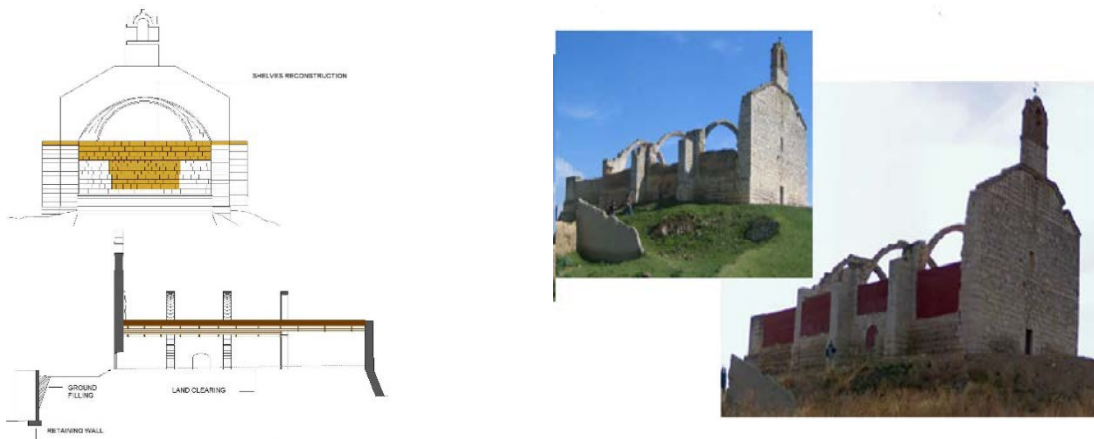
Figure 2. 13: Reconstruction and intervention phase of a damage cultural heritage building. Source: San Jose et al. (2013, p. 371).
