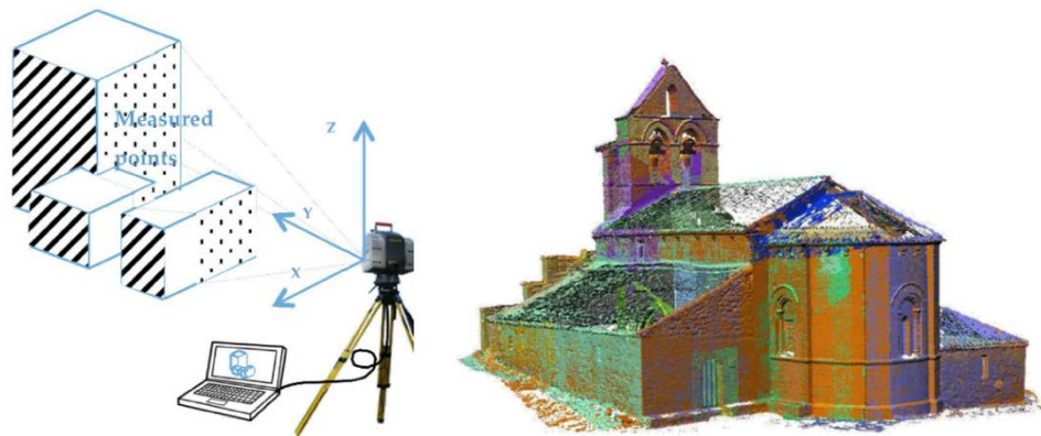
Figure 2. 1 :Laser scanning process to create a point cloud and Georeferenced point cloud, (X, Y, Z). Source: López et al. (2018, p. 8).
