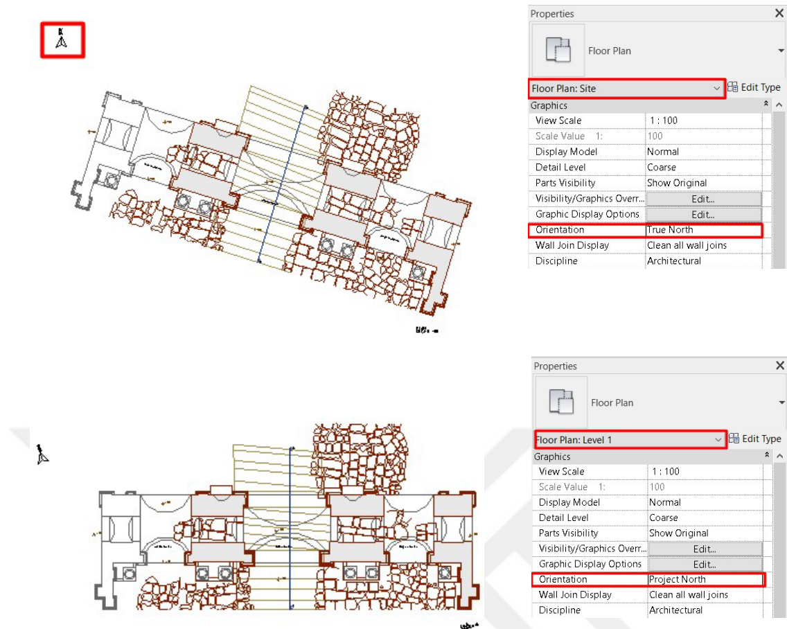
Figure 3. 21: Plan view in true north and project north option. Source: Author's archive.
