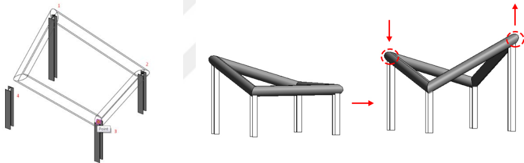
Figure 2. 20: Movement of adaptive points. Source: Molinos (2016).
