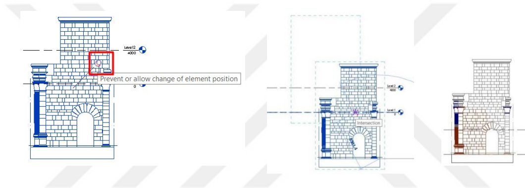
Figure 3. 27: Placing drawing to accurate position. Source: Author's archive.
