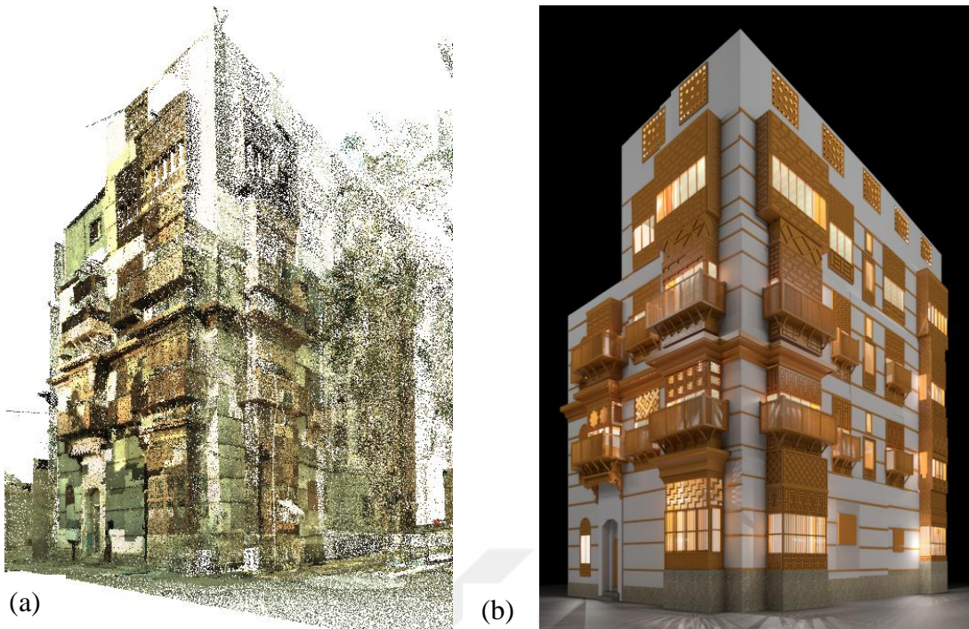
Figure 2. 9: (a) 3D Point cloud model, (b) 3D model by Autodesk Revit. Source: Baik et al. (2013, p. 75).
